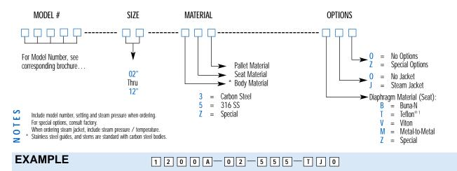
Indicates a 2" Model 1200 with 316 SS Body, Seat and Pallet, Teflon<sup>®1</sup> Seat Diaphragm, Steam Jacketed and no other options.
