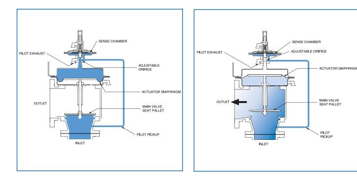
The pilot operated valve is a self-contained system which does not require any external power or pressure source. The pilot valve, using system medium and pressure, automatically controls the actuator pressure to either open or close the main valve depending on the pressure setting of the pilot vs. the actual system pressures.
