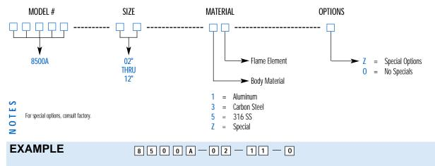
Indicates a 2" Model 8500A with aluminum body, pallet and flame element and no specials.
