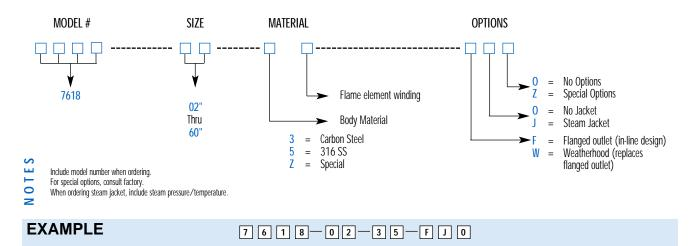
Indicates a 2" Model 7618 with Carbon Steel Body, 316 SS Flame Element Winding, Flanged Outlet, Steam Jacket and no other options.
