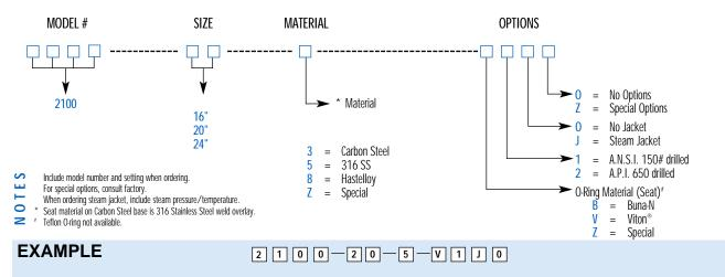
indicates a 20" Model 2100 with 316 SS Material, Viton® Seat O-Ring, ANSI 150# Drilled, Steam Jacket and no other options.
