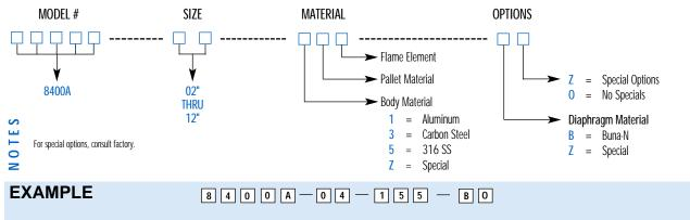
Indicates a 4" Model 8400A with aluminum body, 316SS pallet and flame element, Buna-N diaphragm.
