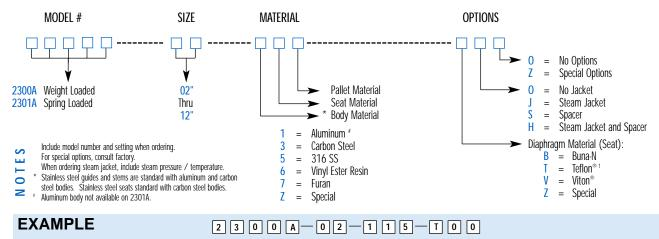
Indicates a 2" Model 2300A with Aluminum Body and Seat, 316 SS Pallet, Teflon®1 Seat Diaphragm and no other options.
