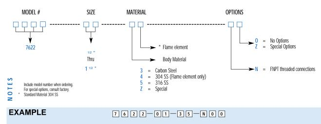
Indicates a 1" Model 7622 with Carbon Steel, 316 SS Flame Element, FNPT connections and no options.
