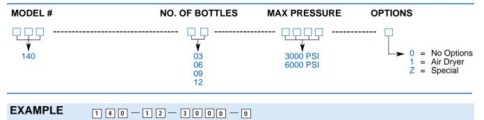
Indicates a compressor with 12 bottles and a maximum pressure of 3000 psi. (as shown in picture on front)
