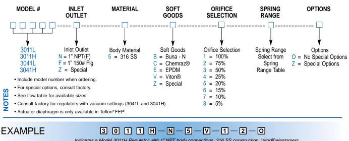
Indicates a Model 3011H Regulator with 1" NPT body connections, 316 SS construction, Vitor®elastomers, full capacity orifice, set pressure range from 1.0" WC to 1.5" WC and no special requirements.
