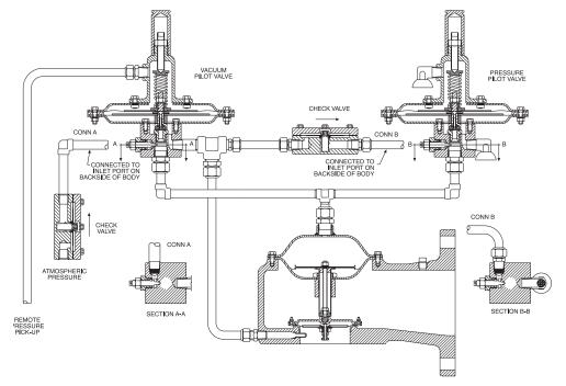
The Model 1663A will be required for pilot operated pressure and vacuum relief when the vacuum setting is greater than the direct actuated vacuum setting of the Model 1661. Minimum vacuum setting for Model 1663A is 3" W.C. and rated capacity is achieved at 10% over-pressure.
