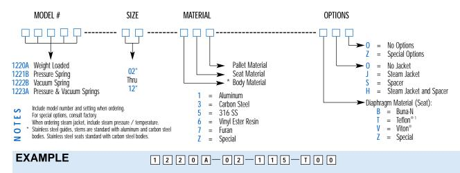
Indicates a 2" Model 1220A with Aluminum Body and Seat, 316 SS Pallet, Teflon®1 Seat Diaphragm and no other options.
