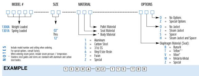
Indicates a 2" Model 1300A with Aluminum Body and Seat, 316 SS Pallet, Teflon®1 Seat Diaphragm and no other options.
