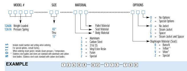
Indicates a 2" Model 1260A with Aluminum Body and Seat, 316 SS Pallet, Teflon®1 Seat Diaphragm and no other options.
