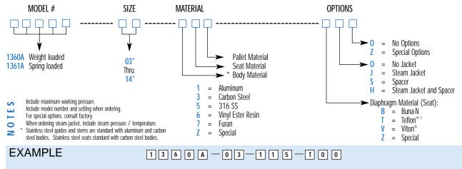
Indicates a 3" Model 1360A with Aluminum Body and Seat, 316 SS Pallet, Teflon®1 Seat Diaphragm , and no other options.
