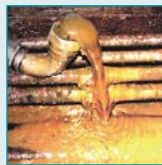
Water Contaminated Oil
